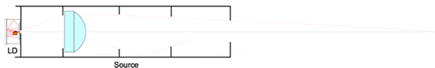
Fig. 13. Baffling of the source.
